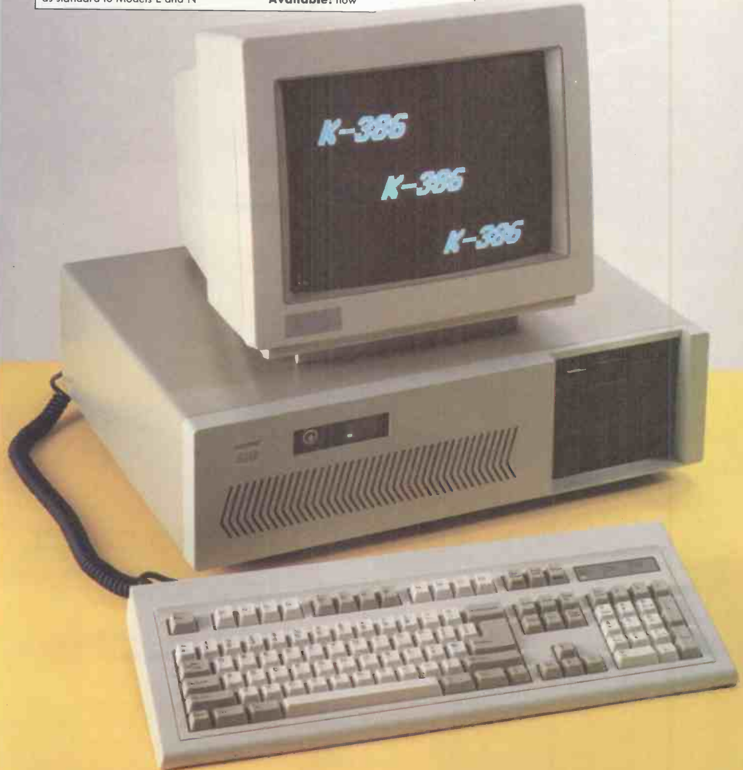
Kaypro has provided three slots to link with its proprietary 32-bit bus. Eight-bit cards will fit but 16-bit AT cards will not.
