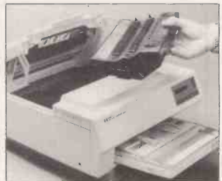
The toner and drum are combined in a single replaceable cartridge.
